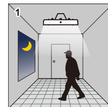
The light switches on at 100% when there is movement detected
